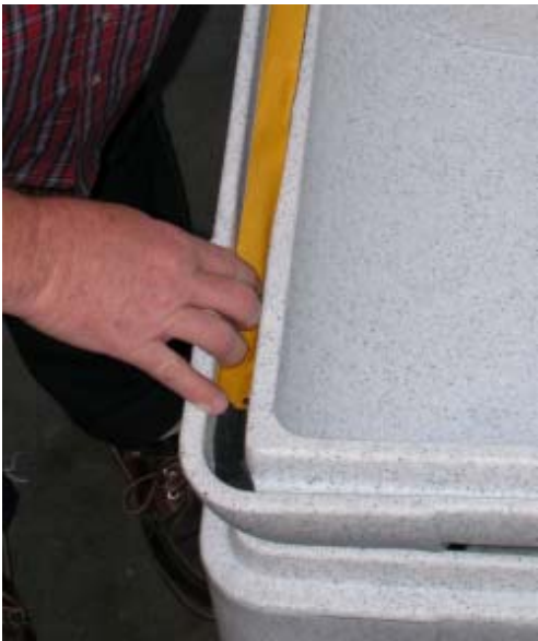
Step 1. Start in one corner and unroll butyl seal pressing seal into groove.
